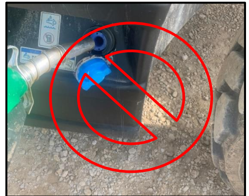
INCORRECT FUEL NOZZLE
